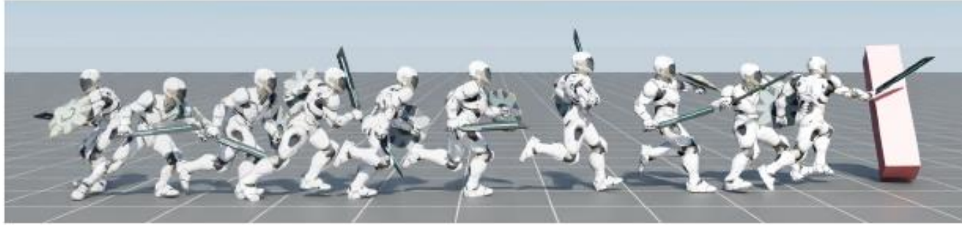
Fig. 1. Our framework enables physically simulated characters to learn versatile and reusable skill embeddings from large unstructured motion datasets, which can then be applied to produce life-like behaviors for new tasks. Here, a character is utilizing behaviors from a learned skill embedding in order to run to a target and knock it over.
